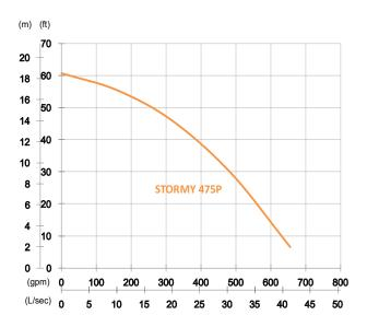
Shaft Speed: 1750 rpm Outlet: 100mm, 4in
